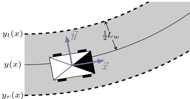
Fig. 2: The robot navigates on the lane of width  $L_w$  modeled as a polynomial equation  $y(x)$ . The left and right borders of the lane are respectively approximated with the polynomials  $y_l(x)$  and  $y_r(x)$ .
