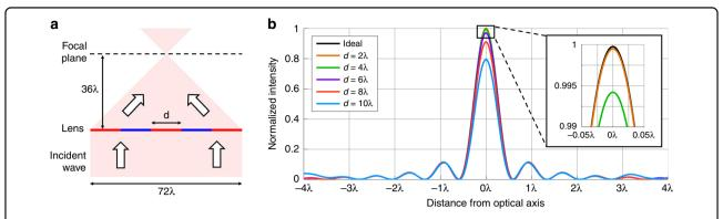
Fig. 2 Impact of phase profile linearization on the cylindrical lens performance. a Cylindrical lenses of focal length 36 $\lambda$  and NA of 0.7 are constructed using linear sections of length d for various values of d. b Line scans of the field intensity at the focal planes of the lenses. Lenses that are linearized with sections that are smaller than 4 $\lambda$  have peak intensities that are within 1% of that of the ideal lens
