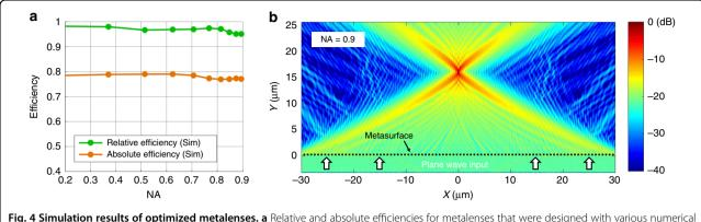
**Fig. 4 Simulation results of optimized metalenses. a** Relative and absolute efficiencies for metalenses that were designed with various numerical apertures. **b** A full-field simulation of a metalens with an NA of 0.9
