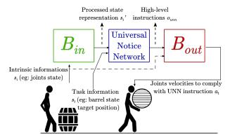
Fig. 3: UNN architecture. The agent receives an observation vector  $s_i$  splitted into a robot observation vector  $s_i$  processed by the input base and a task observation vector  $s_t$ . The UNN, operates on the processed robot information and the task informations. Later the output base, computes the action based on UNN output c and robot intrinsic state vector  $s_i$
