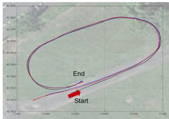
Fig. 4. Ref. path (black), robot traj. with front steering (red) or front and rear steering (blue)
