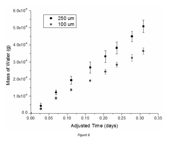
The cumulative lateral permeation as measured by the optical calcium test is shown for all samples. The time axis has been adjusted so that 0 corresponds to the first point after the permeation front had reached the edge of the calcium deposit.
