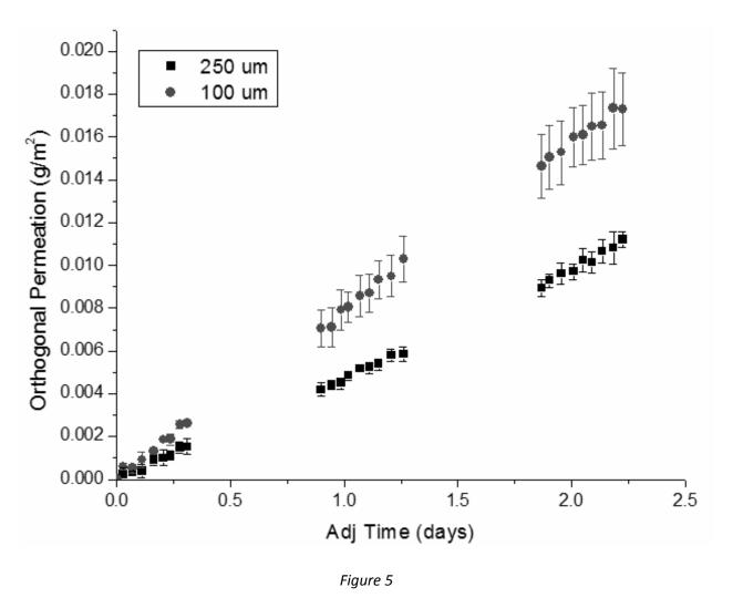
The cumulative water vapor permeation for each sample as measured by the optical calcium test is shown in units of mass of permeated water per unit area. The time axis has been adjusted to remove the effect of residual water in the samples reacting with the calcium at the start of the test. All measures were in the Central Zone of the respective samples and are linear which indicates steady state permeation.
