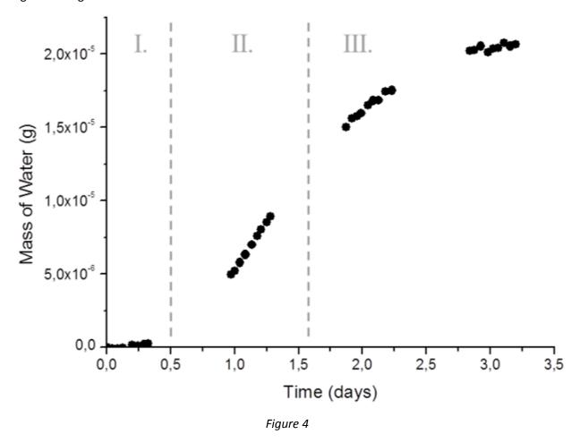
The cumulative lateral permeation as measured by the modified optical calcium test is shown for sample 100-3. Three distinct regions are visible. Region I shows little permeation as the permeation front has yet to reach the edge of the calcium deposit and Region III is invalid due to testing artifacts. Therefore only Region II is used for calculations.
