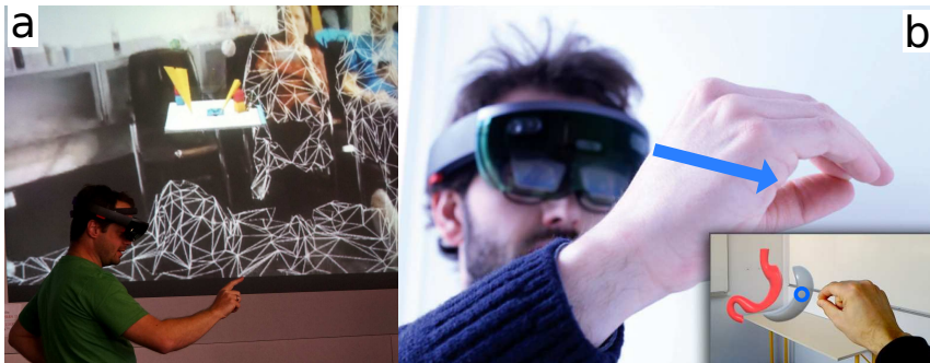
Fig. 3 (a) Example of the environment scanning performed by the HoloLens; it is decomposed in multiple triangles in order to create a 3D model of the scene where possible interactions will be allowed. (b) Photo montage illustrating the user of a HoloLens mixed reality headset and the content as seen by him in his own environment (boxed). The blue circle indicates the HoloLens cursor as seen by the user in the scene. The blue arrow indicates the gaze direction of the user. Subfigure (a) is from [21].
