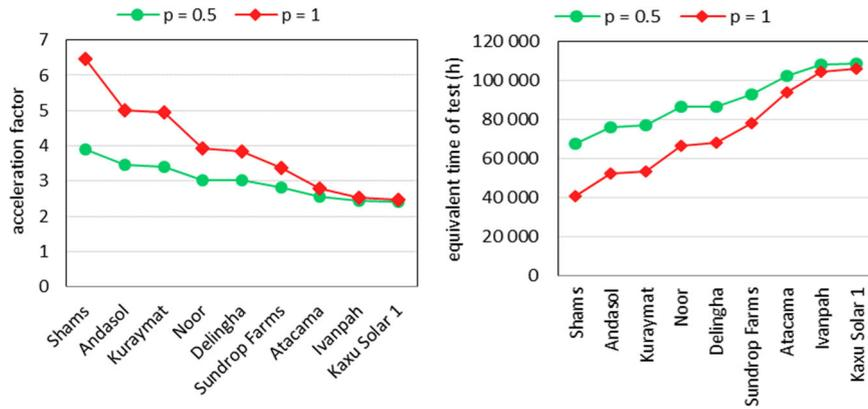
**Fig. 9** Acceleration factors (left) and times of test at 65 W/m<sup>2</sup> equivalent to 30 years on site (right), calculated for 9 sites with  $p = 1$  and  $p = 0.5$  using the annual mean UV irradiance. Site are sorted by increasing irradiance
