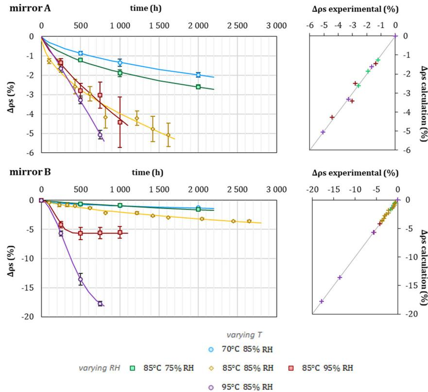
**Fig. 6** Specular reflectance loss of mirrors A and B during damp heat aging tests (left). The marks are the experimental points, and the lines are the extrapolation calculated using Eq. (3). The correlation between the experimental and calculated points is shown on the right side
