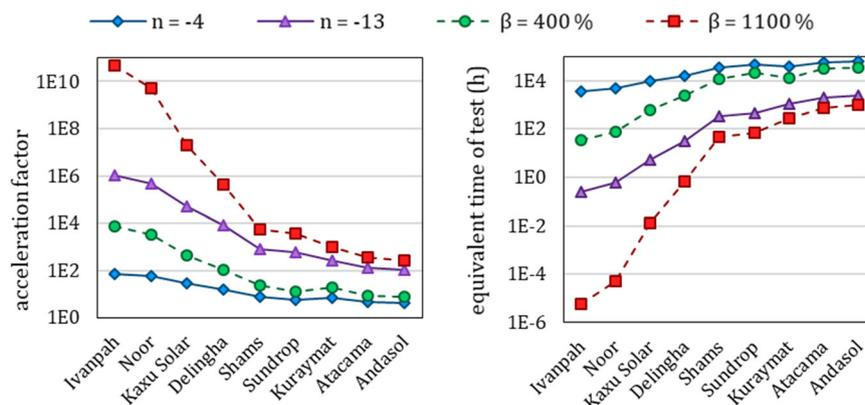
**Fig. 8** Acceleration factors (left) and times of test (right) at 85% RH equivalent to 30 years on 9 sites, with  $n = -4$  or  $-13$  using Peck's model and with  $\beta = 400$  or  $1100\%$  using Eyring's model. Sites are sorted by increasing annual mean relative humidity
