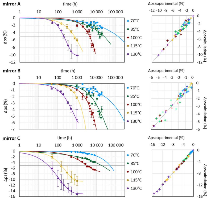
**Fig. 1** Specular reflectance loss of mirrors A, B, and C during temperature aging tests (left). The marks are experimental points, and lines are the extrapolation calculated using Eq. (3). The correlation between experimental and calculated points is shown on the right side
