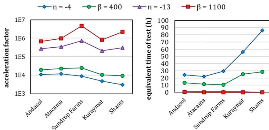
**Fig. 10** Acceleration factors (left) calculated by coupling temperature and humidity and times of test (right) at 85 °C and 85% RH equivalent to 30 years on site, calculated for 5 sites with  $E_a = 100$  kJ/mol and  $n = -4$  or  $n = -13$ ;  $\beta = 400$  or  $\beta = 1100$
