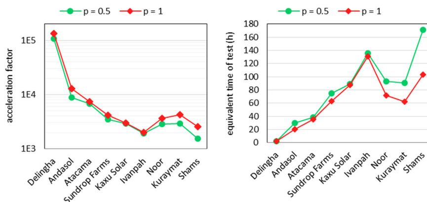
**Fig. 11** Acceleration factors (left) calculated by coupling temperature and irradiance according to Eq. (20) and times of test (right) at 85 °C and 65 W/m<sup>2</sup> equivalent to 30 years on site, calculated for 9 sites with  $E_a = 100$  kJ/mol and  $p = 0.5$  or 1
