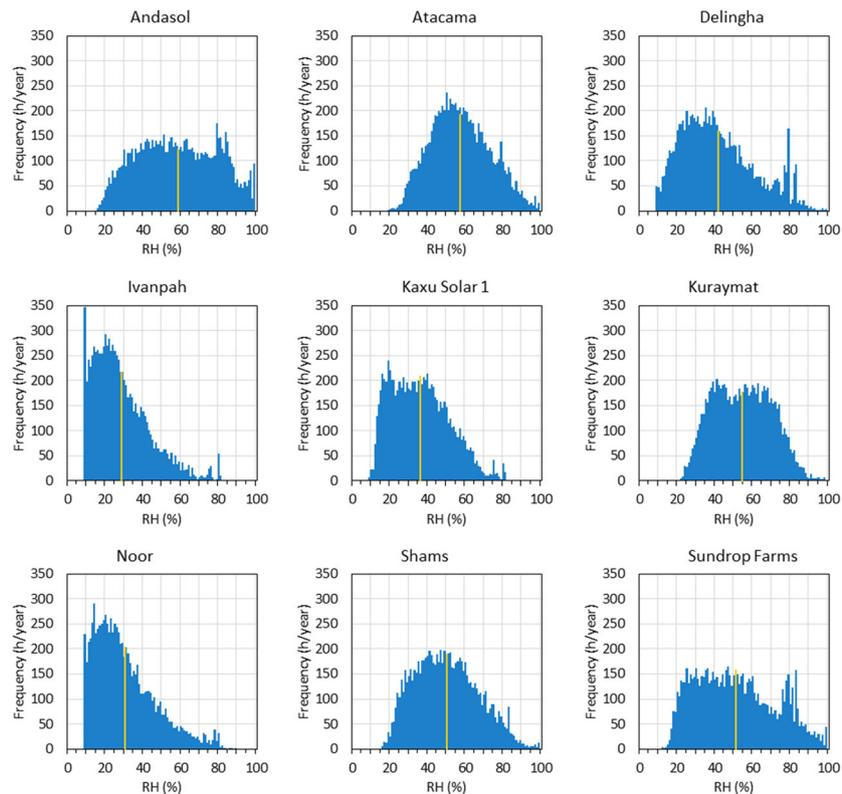
**Fig. 15** Relative humidity frequency in the range 10–100% in hours per year for the 9 sites. The yellow straight line highlights the average annual relative humidity (data obtained from *Meteonorm*<sup>®</sup> 7.2 software (Company, Meteotest *Meteonorm 7: Global Meteorological Database for Solar Energy and Applied Climatology*. (2015)
