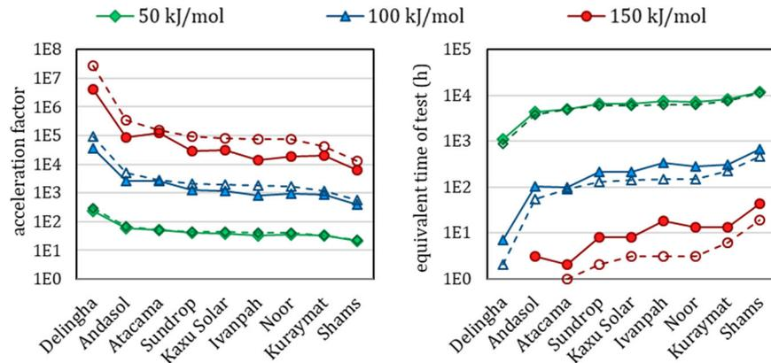
**Fig. 5** Acceleration factor (left) and time of test (right) at 85 °C equivalent to 30 years on 9 sites, calculated with  $E_a = 50, 100$  or 150 kJ/mol using the effective (full lines) or the mean (dash lines) temperature. Sites are sorted by increasing annual mean temperature
