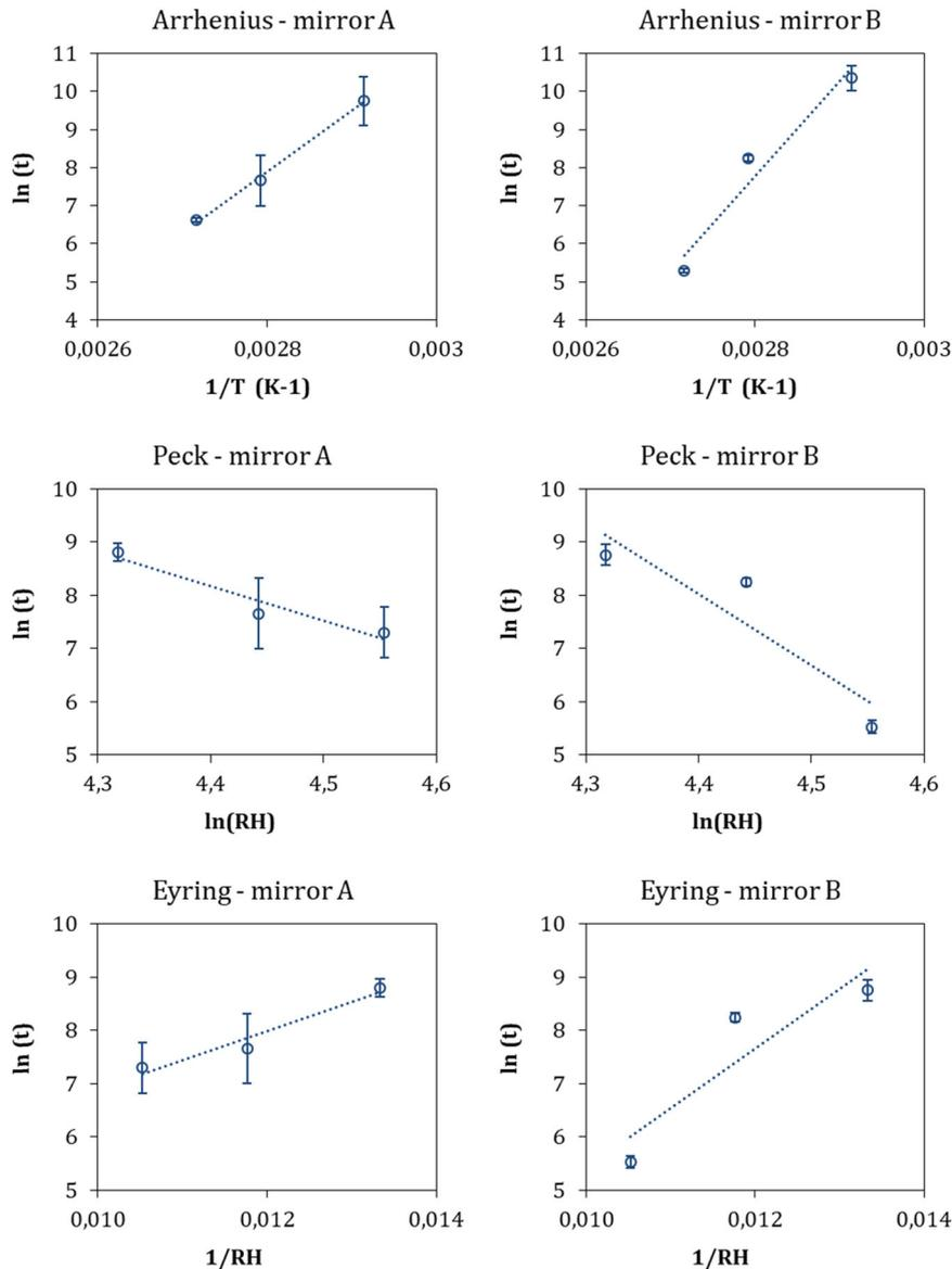
**Fig. 7** Graphical representations based on Arrhenius (top), Peck (middle) and Eyring (bottom) relationships to determine respectively the apparent activation energy in the damp heat test  $E_{a(RH)}$  with RH = 85%, and Peck's parameter  $n$  and Eyring's parameter  $\beta$  with  $T = 85^\circ\text{C}$  for mirrors A and B. Error bars represent the standard deviation of experimental measurements
