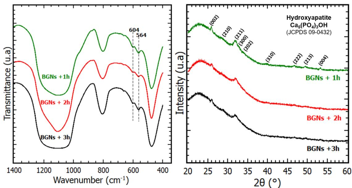
**Figure 6.** IR spectra (right) and XRD patterns (left) of BGNs soaked in SBF for 7 days.
