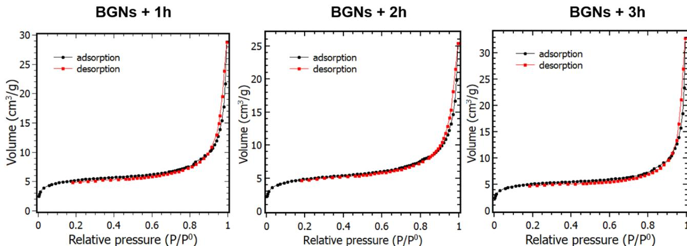
**Figure 2.** Adsorption-desorption isotherms of BGNs+1h, BGNs+2h and BGNs+3h.
