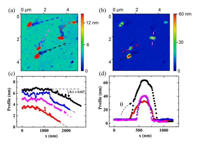
**Figure 6**: (a) AFM images showing the etching of the  $SiO_2$  layer by migration of the Au droplets. The tracks behind the droplets show the Si(111) substrate with the Au-( $\sqrt{3} \times \sqrt{3}$ )-Si(111) surface reconstruction.(b) Same as (a) but with extended height scale to show the droplet morphology. (c)-(d). Height profiles along the dashed lines in (a) and (b), respectively.
