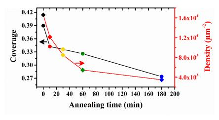
**Figure 4**: Density of droplets and surface coverage as function of the annealing time. The colors of the data points correspond to those used for the distributions in Figure 3.
