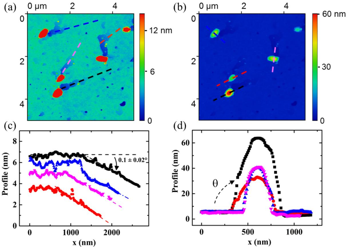
**Figure 6:** (a) AFM images showing the etching of the SiO<sub>2</sub> layer by migration of the Au droplets. The tracks behind the droplets show the Si(111) substrate with the Au-( $\sqrt{3} \times \sqrt{3}$ )-Si(111) surface reconstruction. (b) Same as (a) but with extended height scale to show the droplet morphology. (c)-(d). Height profiles along the dashed lines in (a) and (b), respectively.
