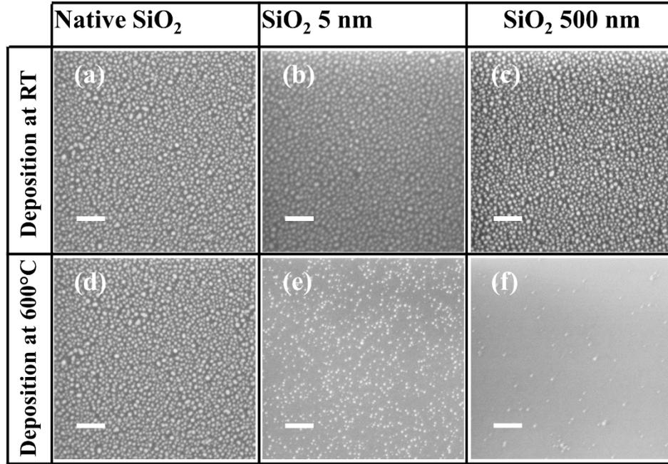
**Figure 1:** SEM images showing the distribution of as-deposited Au after evaporation of 1 nm of Au at RT (upper row) and 600 °C (lower row) on different types of substrate: (a and d) native oxide, (b and e) 5 nm-thick oxide, and (c and f) 500 nm-thick oxide. Scale bar = 100 nm.
