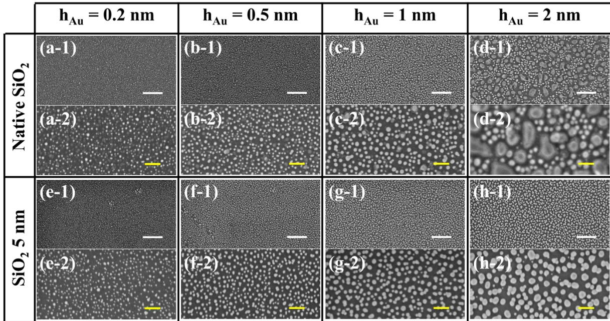
**Figure 2:** SEM images showing the distribution of Au droplets after deposition of (a,e) 0.2, (b,f) 0.5, (c,g) 1 and (d,h) 2 nm of Au at RT followed by annealing at 600 °C for 10 minutes under UHV. The upper two rows correspond to samples with native SiO<sub>2</sub> and the bottom two rows correspond to samples with 5 nm thick thermal oxide. The white and yellow scale bars represent 200 nm and 50 nm, respectively.
