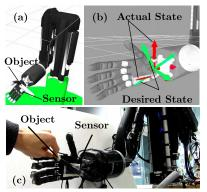
Fig. 12: Edge orientation servoing in the Cartesian space.
