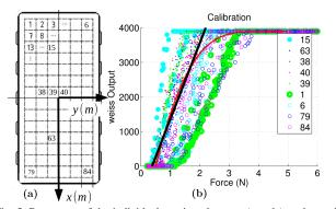
Fig. 5: Responses of the individual sensing elements (tactels) to the applied forces on each element. The sensor outputs are the raw values of the WeissRobotics WTS 0614 sensor that is based on the electro-conductive rubber technology. (a) Locations of tactels and (b) the raw output values of tactels versus ground-truth forces.
