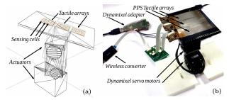
Fig. 10: (a) Experimental platform with  $3 6 \times 4$  DigiTacts Pressure Profile System tactile sensing arrays for validation of a continuously changing tactile image. (b) The real 2dof platform.
