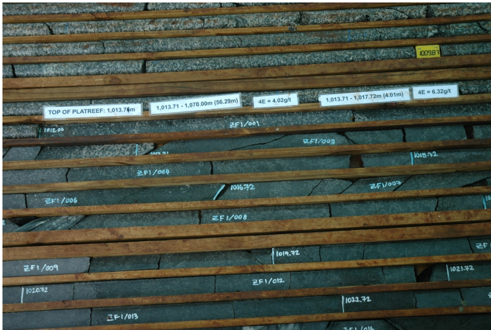
Fig. 6. The contact between norite of the Lower Main Zone and the distinctly more mafic Platreef Unit occurs at a depth of 1013.71 m in drill-hole ZF-1. Average grades of 4.02 g/t over a width of 56.29 m, and 6.32 g/t over a width of 4.01 m, are for 3PGE+Au using base of the Lower Main Zone as datum selected by the mining company.
