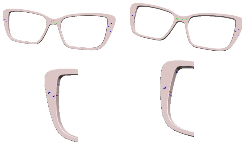
Figure 9: Example of transfert labelling. In light grey it is not labelled face, in blue, it is tenon faces, in green bridge faces and in red circle faces. First line show labelled faces on full mesh and second line is a zoom on the left tenon to show error in labelling process. First column is labelling using transfert with only distance. Second column is labelling using transfert with distance and eigenfunctions.
