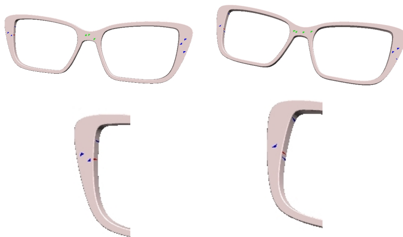
Figure 9: Example of transfert labelling. In light grey it is not labelled face, in blue, it is tenon faces, in green bridge faces and in red circle faces. First line show labelled faces on full mesh and second line is a zoom on the left tenon to show error in labelling process. First column is labelling using transfert with only distance. Second column is labelling using transfert with distance and eigenfunctions.
