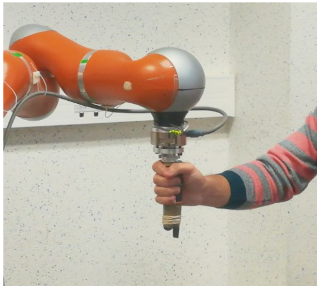
Fig. 1. A cooperative physical Human-Robot Interaction task. The user moves the tool continuously between two points 30 cms apart along a single degree of freedom, using either Impedance or Admittance Control, with a laser pointer attached to the end-effector of the robot. The position and velocity of the end-effector are recorded, as well as the force applied by the human. An RNN with LSTM units is trained over each of the datasets to predict the desired human motion.
