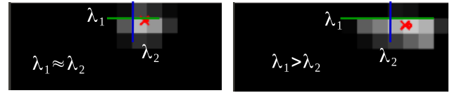
Figure 4: A point-contact type and an edge-contact type on the left-hand and right-hand sides, respectively. The ratio between the lengths of first two principal components in the tactile images are different for these two types of contact.
