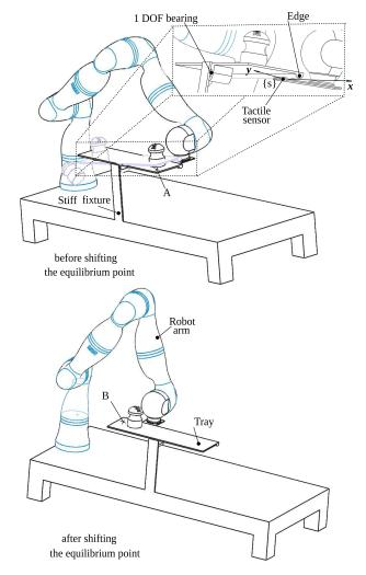
Figure 13: The platform used for balancing a 1 DOF tray in comanipulation task. (Top) The robot arm holding the tray that can rotate around its center thanks to its 1 DOF bearing. If the object on the tray will shift from the initial equilibrium point A, the tray would rotate and the object would fall down (depicted with violet contours). (Bottom) The robot arm performed a corrective motion to keep the tray at its equilibrium state. The center of mass of the tray shifted from point A to B.
