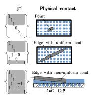
Figure 7: Illustration of elements of the touch-dependent tactile Jacobian for three physical contacts: point, edge, and edge with non-uniform load. The shaded rows in  $\mathbf{J}^{-1}$  of every contact type contribute to the robot end-effector pose.
