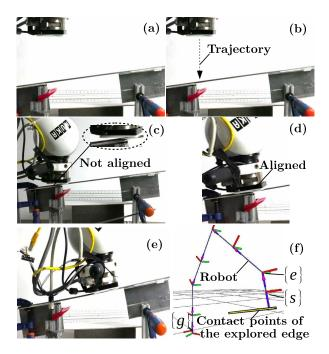
Figure 9: Exploring an unknown shape of a metal bar: align with an edge and move along the detected edge. (a) The initial state. (b) Trajectory that the end-effector follows until (c) it detects a contact. (d) Alignment with an edge. (e) Following the edge. (f) Reconstructed bar at the end of the exploration.
