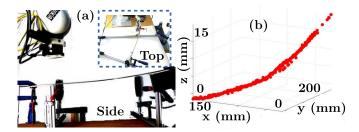
Figure 11: Exploration of a bent bar. (a) The bar and the robot from side and top views. (b) The resulting points of contact of the exploration.
