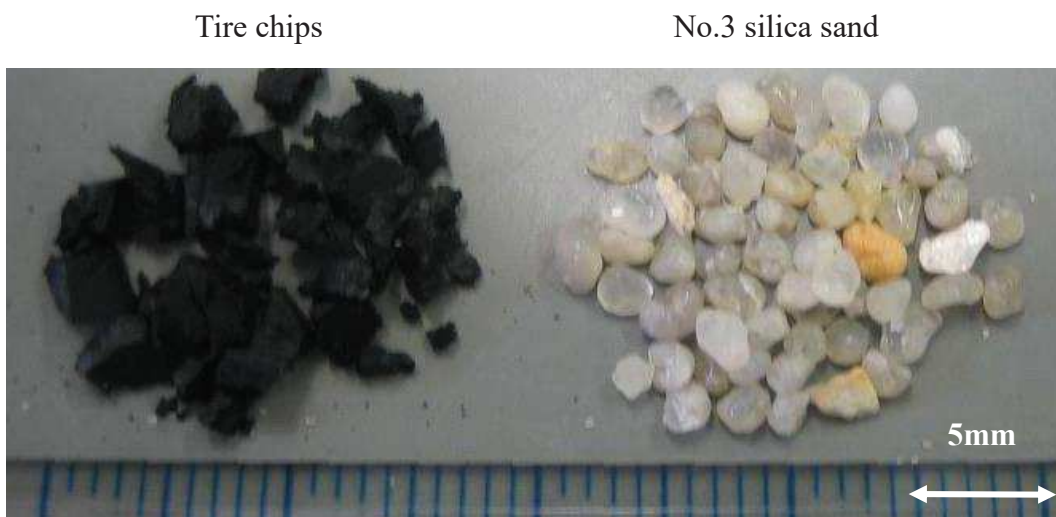
Fig. 4 View of the granular materials tested: tire chips (left) and No. 3 silica sand (right).
