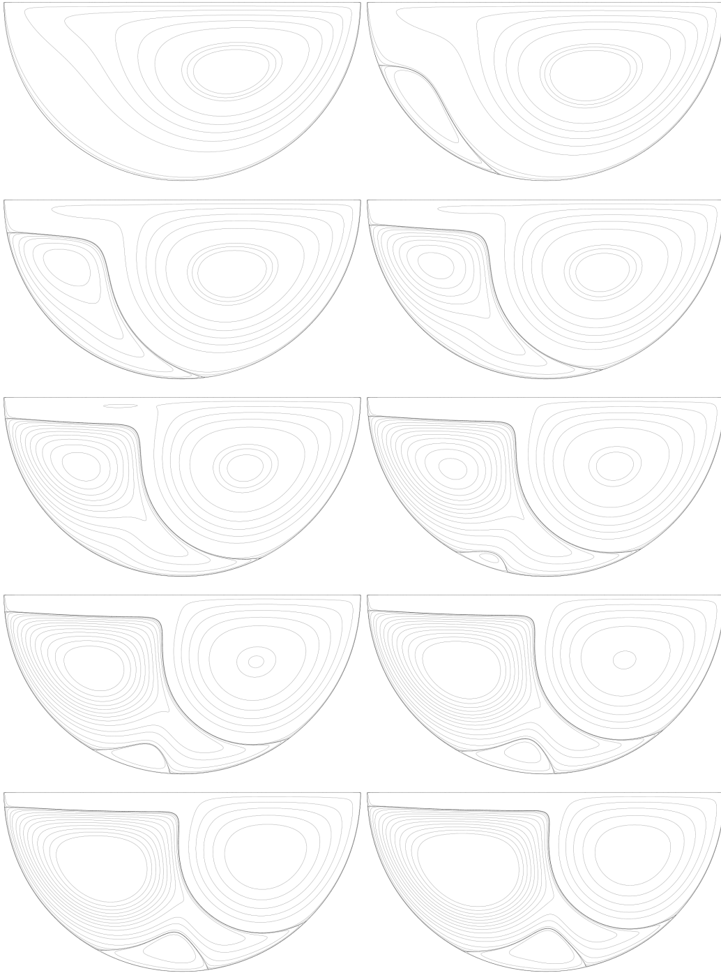
FIGURE 5. Streamlines of the steady state solution for \nu^{-1} = 500, 1000, 2000, 3000, 4000, 5000, 6000, 7000, 8000 and \nu^{-1} = 9000 .
