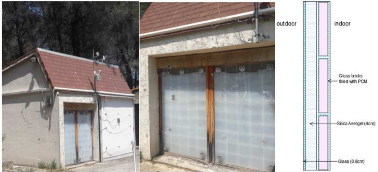
Figure 2: TIM-PCM wall from the outside and Schematic of the TIM-PCM wall composition
