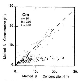
FIG. 16. Comparison of the particle concentration obtained from probe 6 by using two methods of sampling-time determination (A and B) and for the particles larger than  $100~\mu m$  (Cm). The regression parameters are calculated only for measurements having a correct coding of the time parameters. Irregular ice particles were sampled (flight 6), and the airspeed is about 110 m s<sup>-1</sup>.
