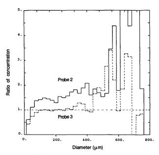
FIG. 13. Ratio of the concentrations P2/P1 and P3/P1 as a function of the diameter, from the same data as to the Fig. 12 results.
