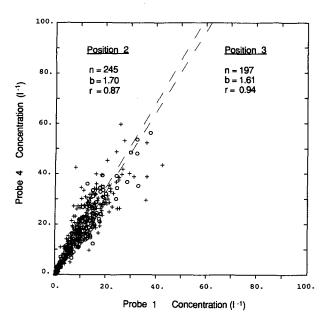
Fig. 3. Comparison of the particle concentration obtained from probe 4 and probe 1. Crosses represent measurements obtained by probe 4 mounted in position 2; circles represents measurements obtained with the same probe mounted in position 3 (see Fig. 2). The symbols n, b, and r refer to the number of data points, the slope of the best-fit curve equation, and the correlation coefficient, respectively.
