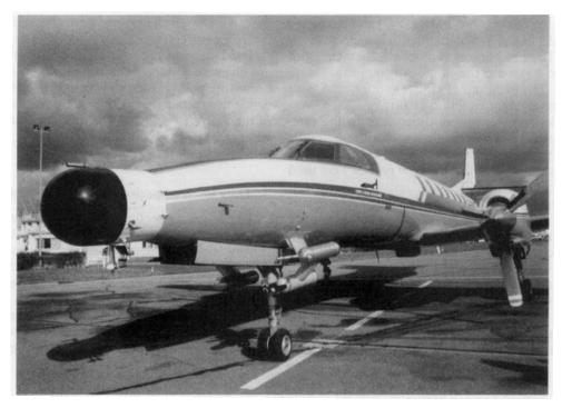
FIG. 1. The Merlin IV of the Centre d'Aviation Météorologique, showing the mounting location for PMS probes beneath the nose. (Courtesy of the French Meteorological Research Center: Météorologie Nationale, EERM/PAD.)
