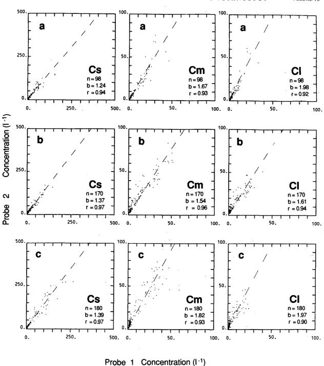
FIG. 9. Comparison of the particle concentrations obtained from probe 2 and probe 1 for the three size ranges already defined, Cs, Cm, and Cl, and three airspeed ranges: (a) from 80 to 90 m s<sup>-1</sup>, (b) from 90 to 110 m s<sup>-1</sup>, and (c) from 110 to 130 m s<sup>-1</sup>. The data were obtained at different levels (+3° to -35°C) in an embedded convective layer (where the particle were drops and ice columns) and then in altostratus and cirrus clouds (irregular ice particles).
