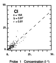
FIG. 8. As Fig. 6 but plotting probe-6 data against data from probe 1. The data were obtained in cirrostratus cloud (bullet rosette ice crystals).
