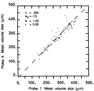
FIG. 14. Comparison of the particle mean volume size obtained from probe 5 and probe 1 at an airspeed of 100 m s<sup>-1</sup>  $\pm$  10%. The data were sampled in a cirrostratus cloud (bullet rosette crystals).
