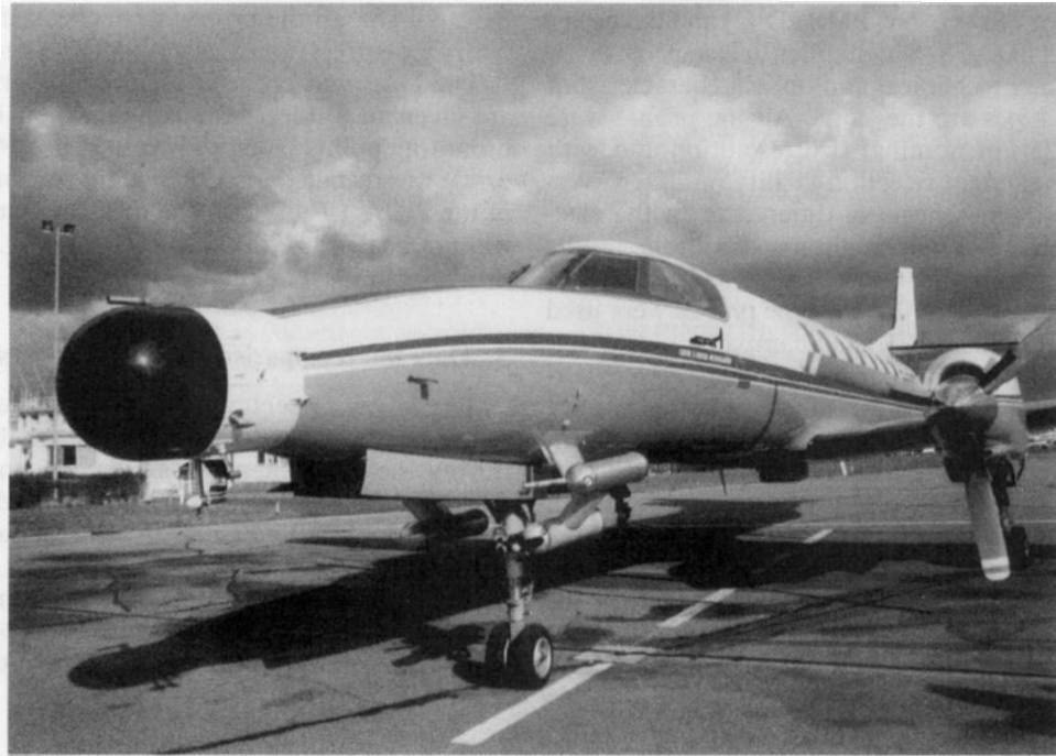
FIG. 1. The Merlin IV of the Centre d'Aviation Météorologique, showing the mounting location for PMS probes beneath the nose. (Courtesy of the French Meteorological Research Center: Météorologie Nationale, EERM/PAD.)
