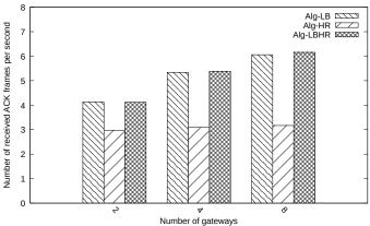
Fig. 8. Number of received ACK frames according to the number of gateways with N=100 end-devices for ENV scenario.
