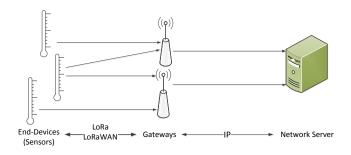
Fig. 1. In LoRaWAN architecture, end-devices communicate to the network server through gateways.
