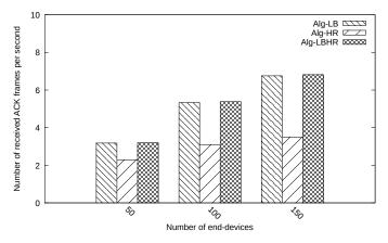
Fig. 7. Number of received ACK frames according to the number of end-devices with g=4 gateways for ENV scenario.
