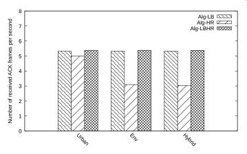
Fig. 6. Number of received ACK frames with N=100 end-devices and g=4 gateways for the three algorithms in each scenario.
