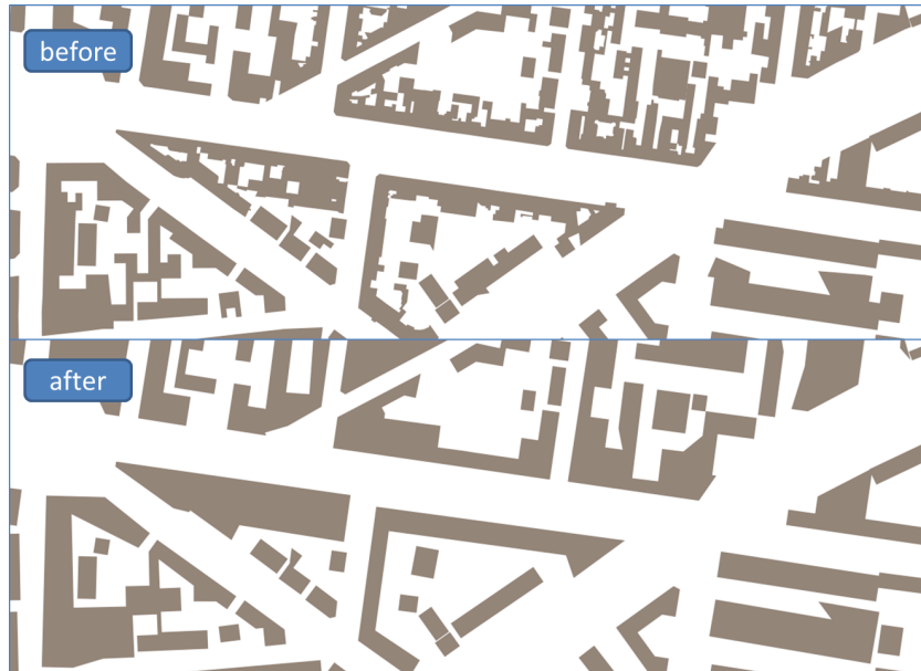
Figure 12: Process used for automatic building generalization.
