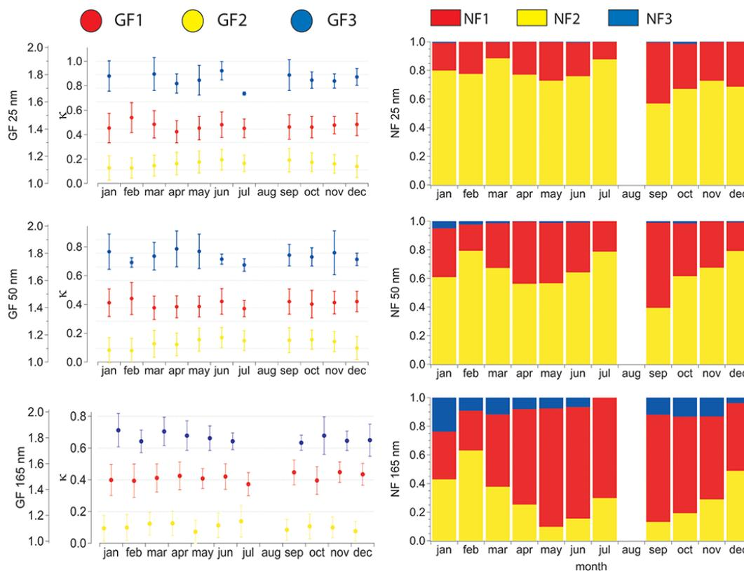
**Figure 5.** Annual variation of hygroscopic growth factor (GF), kappa value ( $\kappa$ ) (left panels) and number fractions (NF) (right panels) measured at RH90 for particles in the nucleation mode (top panels), Aitken mode (middle panels) and accumulation mode (bottom panels). The coloured bars show the average NF of each hygroscopic mode and the markers give the average GF in each mode, including standard deviations.
