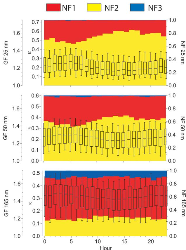
**Figure 6.** Diurnal variation of hygroscopic growth factor (GF), kappa value ( $\kappa$ ) and number fractions (NF) measured at RH90 for particles in the nucleation mode (top panel), Aitken mode (middle panel) and accumulation mode (bottom panel). The figure shows the median GF value, with the bottom and top sides of the box giving the 25th and 75th percentiles, and the extremities the 10th and 90th percentiles. The coloured bars illustrate the NF of particles found in each hygroscopic mode.
