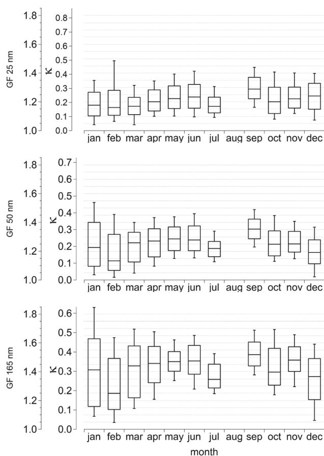
**Figure 3.** Monthly variation of hygroscopic growth factors (GFs) and kappa values ( $\kappa$ ) measured at RH90 for particles in the nucleation mode (top panel), Aitken mode (middle panel) and accumulation mode (bottom panel). The figure shows the median GF and  $\kappa$  value, with the bottom and top sides of the box giving the 25th and 75th percentiles, and the extremities the 10th and 90th percentiles.
