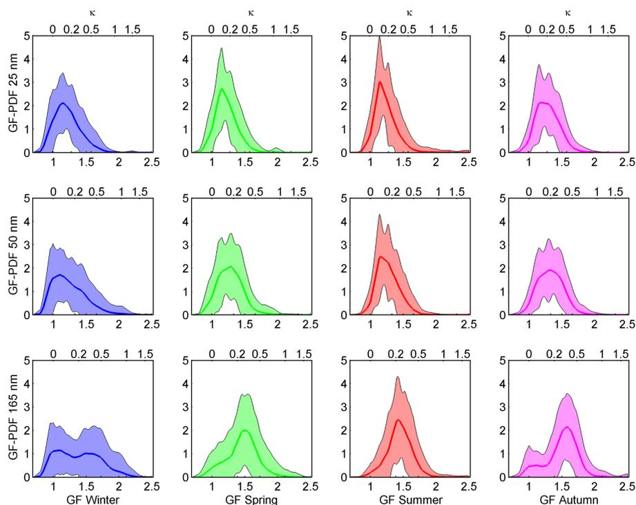
**Figure 4a.** Average GF-PDFs and their standard deviations for particles in the nucleation mode (top panels), Aitken mode (middle panels) and accumulation mode (bottom panels), split by season and measured at RH90. The bottom axis gives the growth factor GF and the top axis shows the corresponding kappa value  $\kappa$ .
