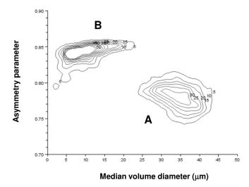
Fig. 5. Mean volume diameter—asymmetry scatter plots of the FSSP-100 and Polar Nephelometer measurements obtained in mixed-phase clouds during ASTAR and POLARCAT experiments ( $\sim 30\,000\,\text{data}$ ). The number of observations are represented by isolines
