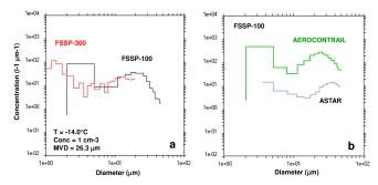
**Fig. 6.** (a): Composite representation of the particle size distributions measured simultaneously by the FSSP-100 and the FSSP-300 in mixed phase clouds during the POLARCAT experiment (12 July 2008). (b): Composite representation of the particle size distributions measured by the FSSP-100 during ASTAR with an air-speed of  $100 \, \mathrm{m \, s^{-1}}$  and during AEROCONTRAIL with an air-speed of  $200 \, \mathrm{m \, s^{-1}}$ .
