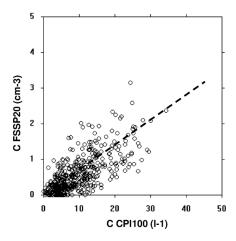
**Fig. 9.** Number concentration of ice crystals  $(d > 20 \,\mu\text{m})$  measured by the FSSP-100 versus the concentration of ice particles  $(d > 100 \,\mu\text{m})$  measured with the CPI (ASTAR, 8 April 2007).
