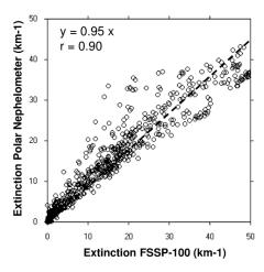
Fig. 2. Relationship between the extinction measurements from the Polar Nephelometer and the FSSP-100. The data correspond to cloud liquid water only (i.e. g > 0.83). ASTAR, 8 April 2007 case study.
