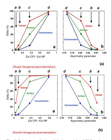
**Fig. 8.** Relative contribution of the ice particles (DELTA values) on number concentration, extinction (surface) and liquid/ice water content (volume) measurements as a function of: the REX extinction ratio (CPI data to PN measurements) and the asymmetry parameter, respectively. The data have been obtained during the cloud sequences labelled a, b, c and d (see Fig. 1). **(a)** Rough hexagonal crystals simulation. **(b)** Smooth hexagonal crystals simulation.
