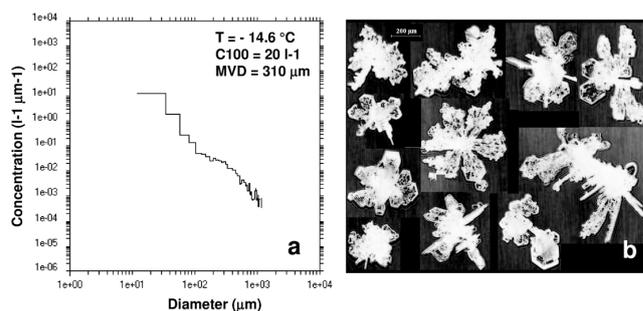
**Fig. 10.** (a) Particle size distribution measured by the CPI during the sequence between 10:58 and 11:06 UTC on Fig. 1 ( $T = -14.6 \text{ }^\circ\text{C}$ ). (b): Examples of ice crystal images measured by the CPI during this sequence.
