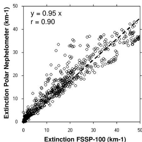
**Fig. 2.** Relationship between the extinction measurements from the Polar Nephelometer and the FSSP-100. The data correspond to cloud liquid water only (i.e.  $g > 0.83$ ). ASTAR, 8 April 2007 case study.
