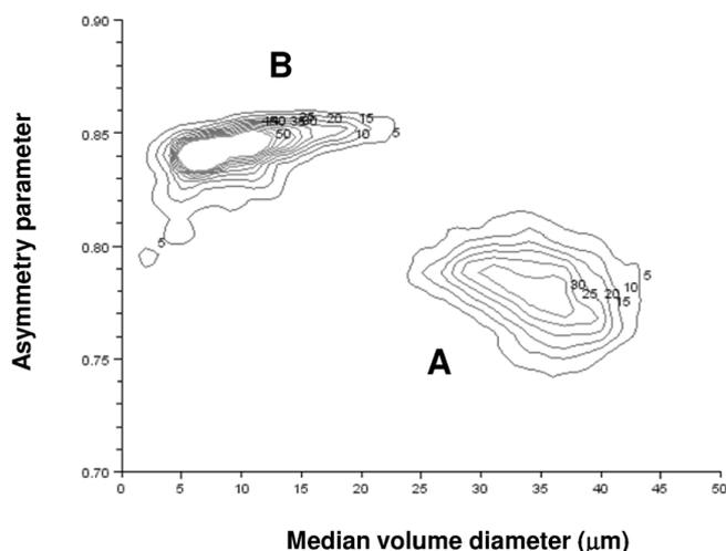
**Fig. 5.** Mean volume diameter–asymmetry scatter plots of the FSSP-100 and Polar Nephelometer measurements obtained in mixed-phase clouds during ASTAR and POLARCAT experiments ( $\sim 30\,000$  data). The number of observations are represented by iso-lines.
