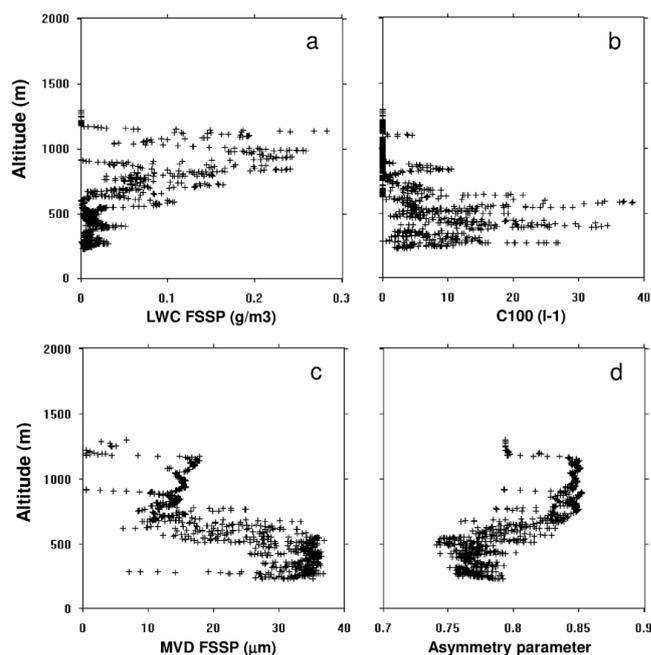
**Fig. 3.** Vertical profiles of cloud parameters obtained during the descent-climbing sequence on Fig. 1. (a): Liquid water content; (b): Concentration of ice particles with  $d > 100 \mu\text{m}$ ; (c): Mean volume diameter and (d): Asymmetry parameter.
