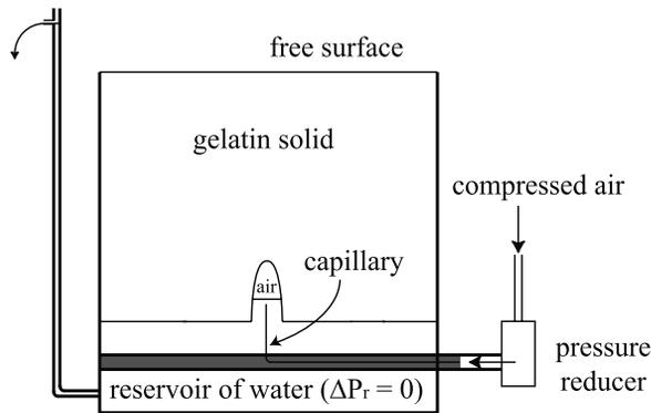
**Figure 1.** Schematic diagram of the experimental apparatus used for the determination of the gelatin fracture toughness. The excess of water is bled off the reservoir while air is injected in the crack insuring a free surface condition at the interface between the water reservoir and the gelatin solid.
