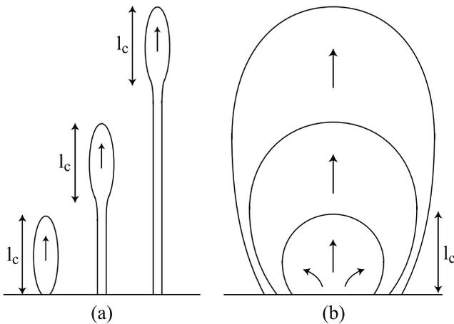
**Figure 11.** Schematic illustration of the fissure propagation in the steady state regime in cross section (a) and in plane (b) views. Once the fissure reaches a height  $l_c$ , the hydrostatic pressure and the source pressure become comparable. Then, the fissure propagates mainly vertically and develops a bulbous head of length  $l_c$ . The propagation is controlled by the balance that takes place in the fissure head between the hydrostatic pressure and the fracture pressure.
