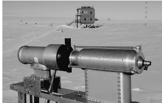
FIG. 1. CPI (right) and PN (left) installed in tandem at the Amundsen–Scott South Pole station during the SPICE experiment.
