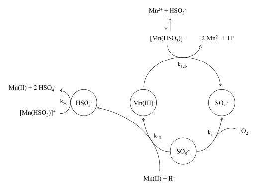
Figure 13. Proposed mechanism for the manganese(III/II)-catalyzed autoxidation of hydrogen sulfite. Reprinted with permission from ref 130. Copyright 1995 Elsevier Science and Technology (http://www.elsevier.com).
