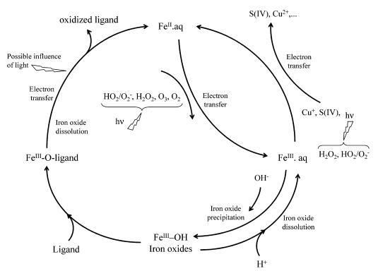
**Figure 8.** Reaction scheme for iron(II)/iron(III) in the dark and/or in the presence of light for atmospheric water. Reprinted with permission from *Nature* (http://www.nature.com), ref 25. Copyright 1990 Nature Publishing Group.
