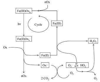
**Figure 12.** Scheme for the photochemical/chemical cycling of iron and formation of  $H_2O_2$ . Reprinted with permission from ref 180. Copyright 1992 American Chemical Society.
