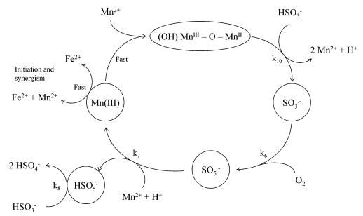
Figure 14. Revised mechanism for the manganese(III/II)-catalyzed autoxidation of hydrogen sulfite. Reprinted with permission from ref 131. Copyright 1998 American Chemical Society.
