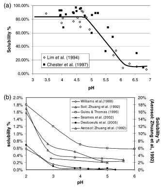
**Figure 1.** pH-solubility relationships for (a) copper in excess of its crustal abundance in rainwaters (the line represents the estimated pH absorption edge) and for (b) iron derived from dust dissolution during leaching experiments.
