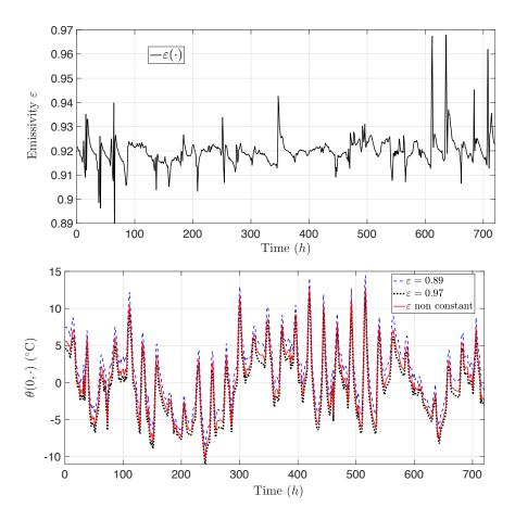
Figure 5: Measurements over one month of the emissivity  $\varepsilon$  (top) and the road surface temperature  $\theta(0,\cdot)$  for the time-dependent  $\varepsilon$ , and constant  $\varepsilon$ 's respectively fixed to the minimal and maximal values (bottom).
