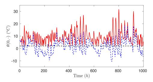
Figure 13: Temperature  $\theta(0,\cdot)$  at the road surface on [0,1000] corresponding to the source q defined by (5.53).
