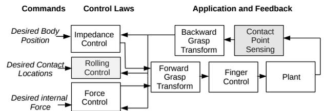
Figure 23: General control framework for dexterous manipulation [157]. The path of information from command through control laws to application on the dexterous hand using object impedance control for rolling manipulation is shown. The highlighted blocks can be replaced with tactile servoing control laws.
