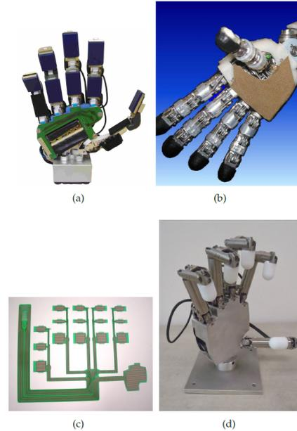
Figure 15: Five-fingered robot hands with tactile sensors: (a) the fluidic robot hand with combined piezoelectric and piezoresistive tactile sensors that can sense high-frequency vibrations due to the absence of electric motors [24], (b) the robot hand of the iCub humanoid robot with tactile sensors on the fingertips and the palm [44], (c) flexible tactile sensing arrays of the SKKU robot hand [88], (d) the SKKU robot hand [88]
