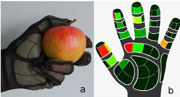
Figure 13: Tactile data glove based on conductive rubber (a) and the tactile information from the data glove during a grasp (b) [54].
