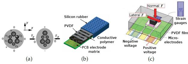
Figure 3: Piezoelectric Tactile Sensing: (a) the piezoelectric effect – an applied force causes rearrangement of positive  $Si$  and negative  $O_2$  particles leading to an increase of potential [45]; (b) a tactile sensing array based on the piezoelectric effect with electrodes on the bottom layer, piezoelectric material in the middle and rubber on the top [24], (c) schematic model of a piezoelectric sensing tactel [71].
