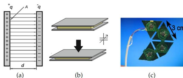
Figure 2: Capacitive Tactile Sensing Technology: (a) capacitance of a parallel plate capacitor depends on distance between plates  $d$  and area of the plates  $A$  ( $q$  is the stored charge) [45]; (b) two conductive plates are separated by an elastic dielectric – as force is applied, the distance between the plates reduces, changing the capacitance [9]; (c) mesh of triangle shape capacitive sensors for the palm of the iCub humanoid robot [44].
