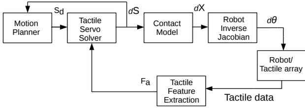
Figure 24: Architecture of a tactile servoing controller [158]. The tactile feature extraction processes the contact information and provides features to control. Desired contact state,  $S_d$ , is compared with the actual contact state,  $S_a$ .  $S_a$  is derived from actual tactile feature,  $F_a$ . The errors in the contact state space are transformed to the joint space of a robot.
