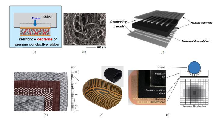
Figure 1: Piezoresistive Tactile Sensor Arrays: (a) illustration of resistance changes in conductive rubber [47],(b) nano-scale image of conductive rubber [48], (c) structure of piezoresistive tactile array [49], (d) piezoresistive fabric tactile sensor [50], (e) schematic of electrode layer of the 3D-shaped tactile sensor [34], (f) tactile image of a piezo-resistive pressure sensor array [35].
