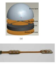
Figure 4: Quantum Effect Tactile Sensing: (a) structure of a tactel of the QTC based tactile sensing array with capability of measuring shear and normal forces [72]; (b) the flexible tactile sensing array for a finger of an anthropomorphic robot hand with the tactels that can measure shear forces [72].
