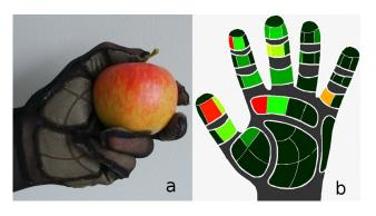
Figure 13: Tactile data glove based on conductive rubber (a) and the tactile information from the data glove during a grasp (b) [54].
