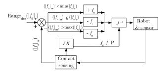
Figure 26: Surface contour following using the contact sensing finger (control diagram). [160].  $Range_{des}(|f_d|_r)$  is a range of the desired force,  $(|f_n|_m)$  is the measured normal force,  $(|f_n|_r)$  is the friction cone,  $(f_n)$  and  $(f_t)$  are the normal and tangential forces, P is the contact point location, and  $(J^{-1})$  is the robot's inverse kinematics.
