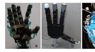
Figure 10: Simple integration of tactile sensing arrays: (a) the Tekscan tactile sensing system consisting of 349 taxels with the Shadow robot hand [94], (b) the Allegro robot hand with PPS RoboTouch capacitive arrays [64], (c) the Robotiq adaptive gripper with sensor suite installed on the contact surface [65]
