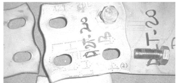
Fig. 3 Zones of deformation (a); joint with two bolts in shear showing large hole elongation after test (b)
