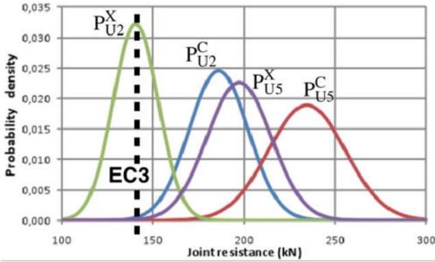
Fig. 10 Probability distributions of the cover-plate joint resistances
