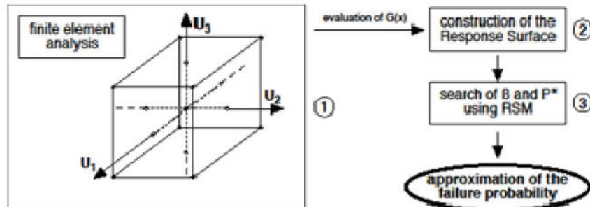
Fig. 7 Analysis procedure in the reliability evaluation
