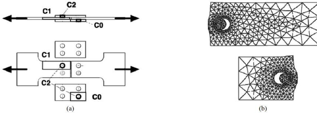
Fig. 4 Cover-plate joint components for modeling (a); deformed components C0 and C1 (b)
