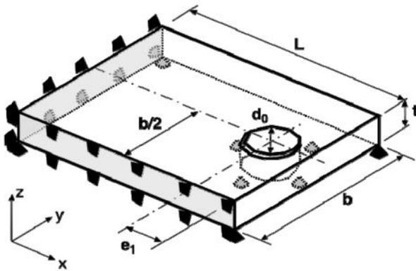
Fig. 8 Geometrical parameters of the plate used in reliability analysis
