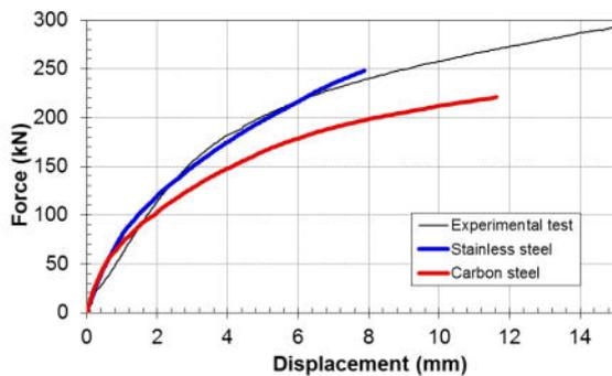
Fig. 5 Load displacement result for 2T-20 joint
