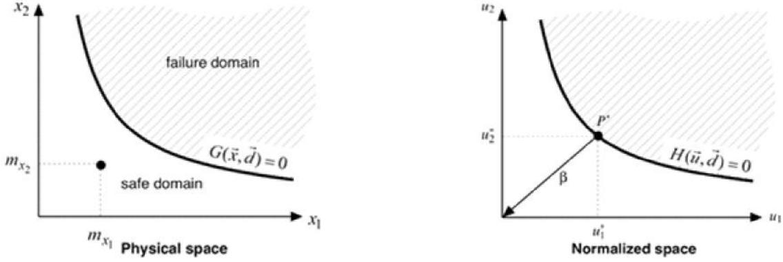
Fig. 6 Physical and normalized spaces for reliability analysis
