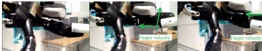
Figure 9: Experiment with the servo-tactile control. Controlling magnitude and position of the force in the contact.
