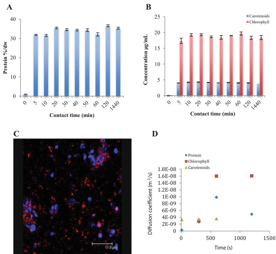
Fig. 5. Assessment of high-pressure homogenization. A – Percentage of hydro-soluble protein concentration per dry weight of biomass. B – Quantification of pigments released in the aqueous phase. C – Microscopic observation of the cells after cell disruption treatment. D – Evolution of proteins and pigment diffusion coefficients in terms of extraction time.
