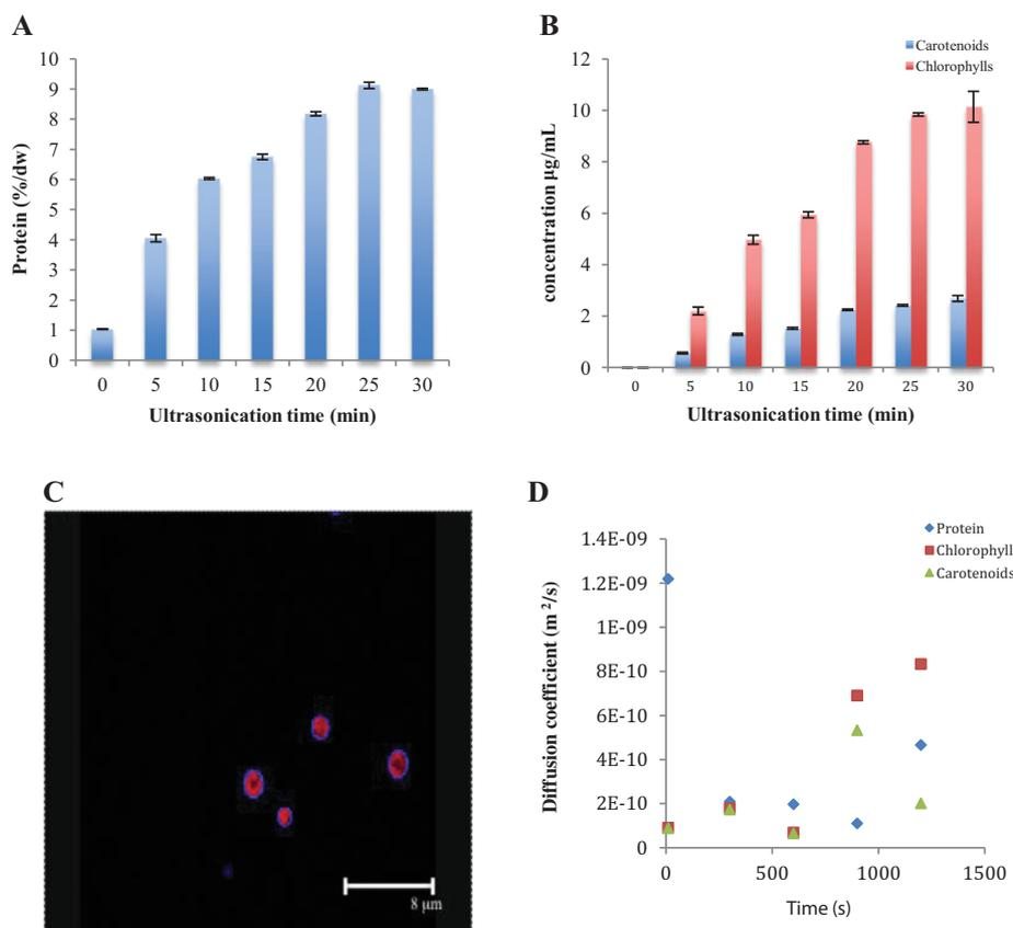
**Fig. 3.** Assessment of ultrasonication. A – Percentage of hydro-soluble protein concentration per dry weight of biomass. B – Quantification of pigments released in the aqueous phase. C – Microscopic observation of the cells. D – Evolution of proteins and pigment diffusion coefficients in terms of extraction time.
