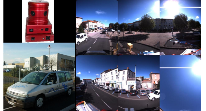
Figure 6: Cameras (PointGrey Ladybug 2) and images for CC. The cameras are global shutter. The camera pointing toward the sky is not used in experiments.
