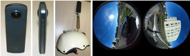
Figure 5: Spherical camera (Ricoh Theta S) and image for WU. Both rolling shutter and image motion go from bottom to top ( \tau is negative, the bottom line is the oldest).
