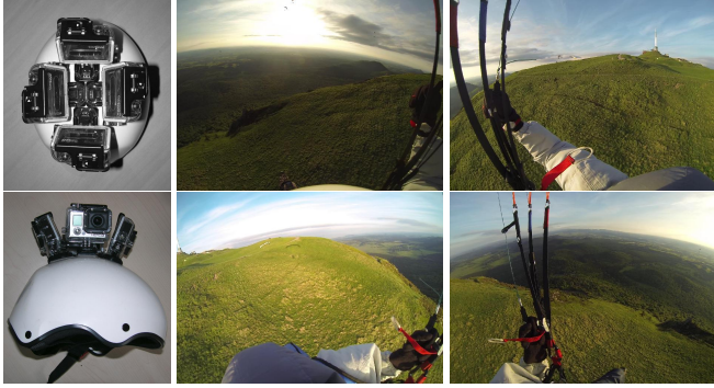
Figure 4: Cameras (four Gopro Hero 3 in their housings) and images for FH. The rolling shutter always goes from top to bottom, the image motion goes forward/toward right/backward/toward left.
