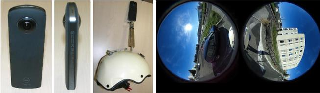
Figure 5: Spherical camera (Ricoh Theta S) and image for WU. Both rolling shutter and image motion go from bottom to top ( $\tau$  is negative, the bottom line is the oldest).
