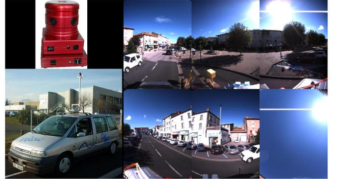
Figure 6: Cameras (PointGrey Ladybug 2) and images for CC. The cameras are global shutter. The camera pointing toward the sky is not used in experiments.
