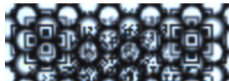
Figure 2. Zoom on a plenoptic raw image.
