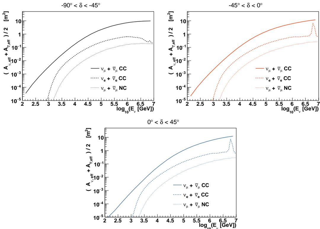
Figure 1: Effective area for  $\nu_\mu + \bar{\nu}_\mu$  CC events after the track selection cuts (solid line) and for  $\nu_e + \bar{\nu}_e$  CC and  $\nu_\mu + \bar{\nu}_\mu$  NC events after the shower selection cuts (dashed lines) considering three declination ranges.
