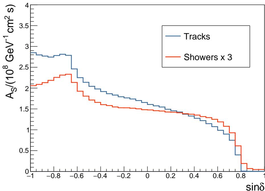
Figure 5: The acceptance as a function of the source declination for an  $E^{-2}$  energy spectrum with a flux normalization factor of  $\Phi_0 = 10^{-8} \text{ GeV cm}^{-2} \text{ s}^{-1}$  for the track (blue) and shower (red) samples. For better visibility, the acceptance for showers is scaled up by a factor 3.
