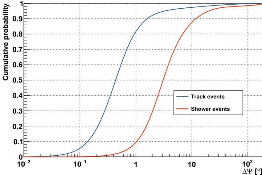
Figure 3: Probability to obtain a reconstructed angle within  $\Delta\Psi$  between the reconstructed direction of track-like events (blue) and shower-like events (red) with respect to the true Monte Carlo neutrino direction. A neutrino flux with an  $E^{-2}$  energy spectrum is assumed.
