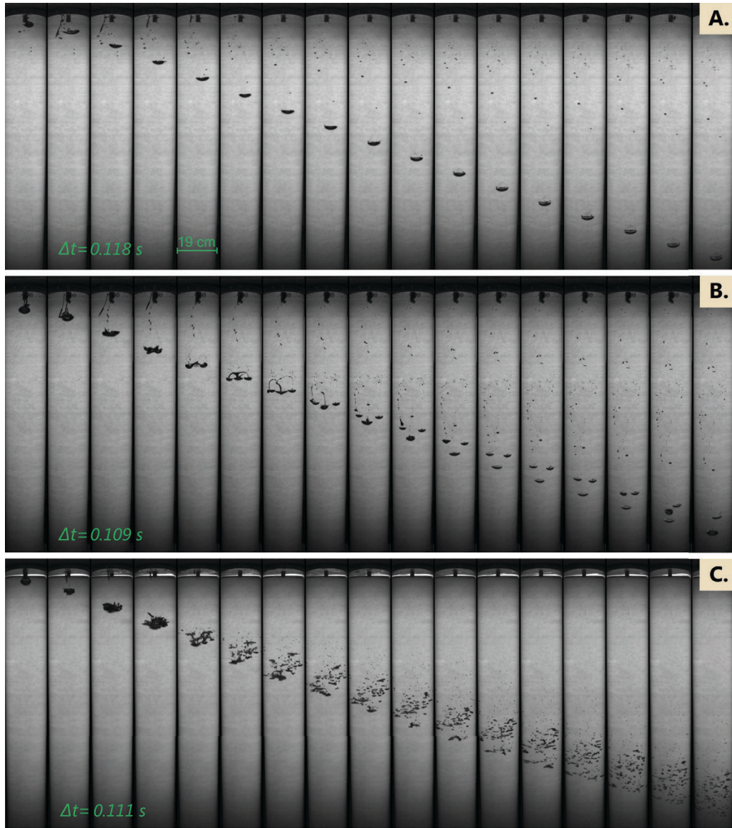
Figure 3: Successive snapshots with a fixed time interval for 3 experiments. A : Fall of a 14 mm initial radius diaphragm in pure glycerine, corresponding to Re_a = 12 , We_a = 14 and a viscosity ratio of 500. The diaphragm has a stable cap shape. B : same as A but for a 23 mm initial radius diaphragm, corresponding to Re_a = 24 and We_a = 37 . The diaphragm breaks up in 3 main cap-shaped stable drops of close sizes. C : same as B but for an ambient fluid 100 times less viscous, corresponding to Re_a = 2400 , We_a = 37 and a viscosity ratio of 5.
