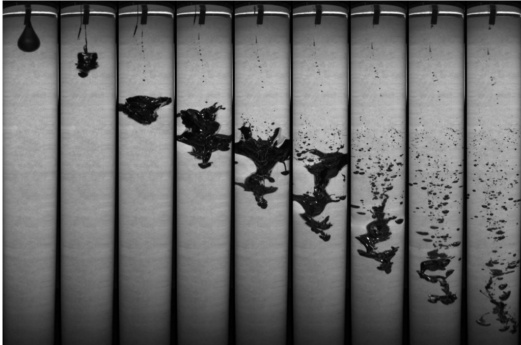
Figure 4: Successive snapshots with a fixed time interval \Delta t = 0.18s for a 30 mm initial radius diaphrag falling through pure glycerol, corresponding to Re_a = 37 , We_a = 64 and a viscosity ratio of 500. One can notice that the mean speed of the front of the diaphrag is rather constant.
