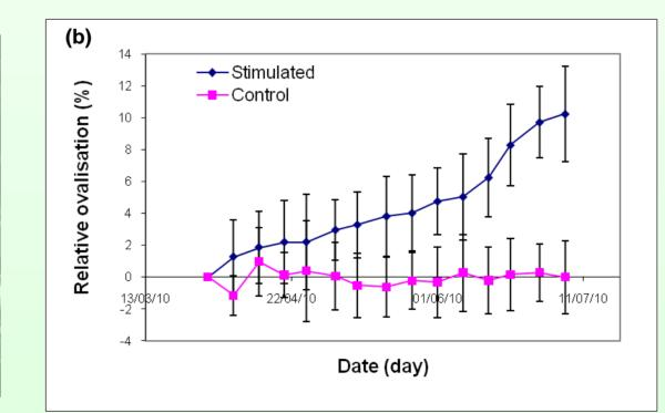
Cambial activity induced by local applied the strains to stem: experimentations and modelling. Plants were subjected to 3 successive daily bendings per week during 4 months. (a) Transversal section of a stimulated plant. (b) Relative ovalisation induced by bending. (c) Strain field for living tissues. (d) Weekly growth rate measurements (blue lines) and growth rate modeling (red lines).
