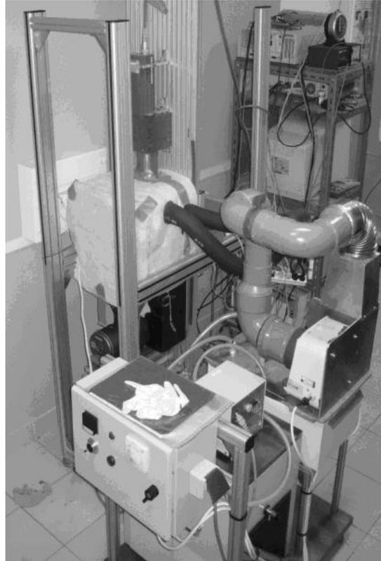
Fig. 1: Principle of the 2D X-ray imaging device and general view of the experimental device (the X-ray imaging system is coupled with the air conditioner).
