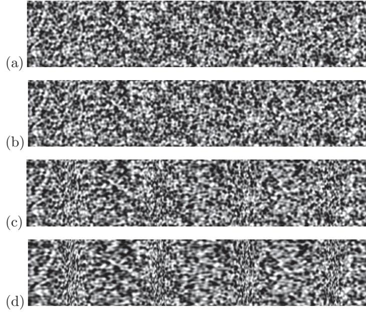
Figure 1: Example of simulated synthetic images: reference (a) and deformed images ( $p = 130$  pixels, (b)  $\alpha = 0.02 - u_{,X}^{Max} = 12.6\%$ , (c)  $\alpha = 0.05 - u_{,X}^{Max} = 31.4\%$  and (d)  $\alpha = 0.1 - u_{,X}^{Max} = 62.8\%$ ).
