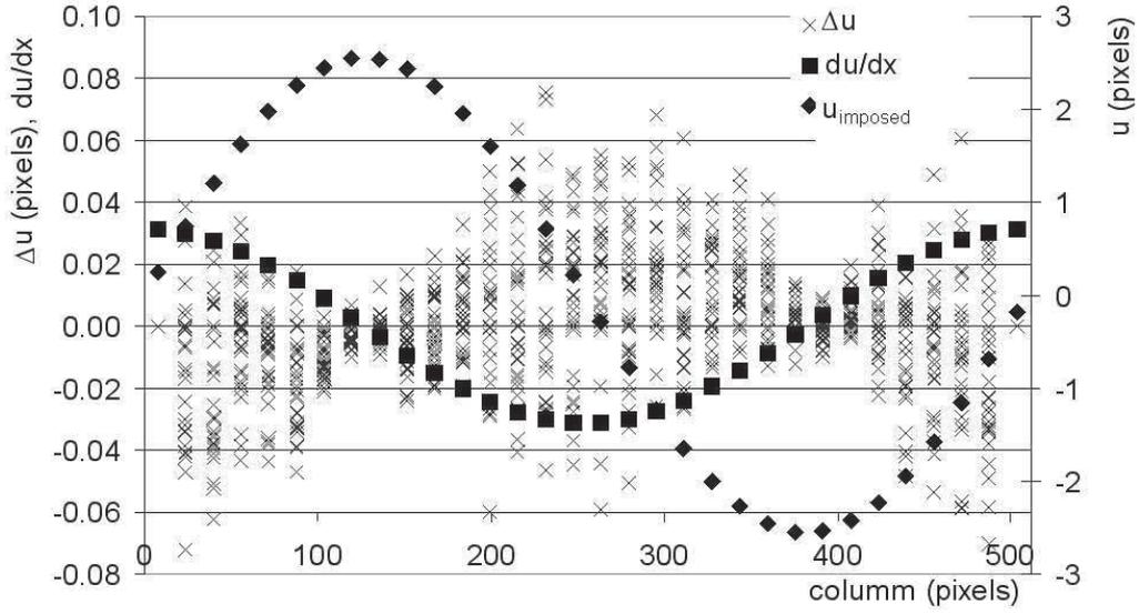
Figure 6: Imposed displacement, displacement gradient and local error  $\Delta u(i, j)$  as a function of the column of the image ( $\alpha = 0.005$ ,  $p = 510$  pixels,  $d = 16$  pixels, zero order shape function  $\Phi$ ,  $u^{Max} = \alpha p = 2.55$  pixels, and  $\left(\frac{du}{dx}\right)^{Max} = u_{,X}^{Max} = 2\pi\alpha = 3.1\%$ ).
