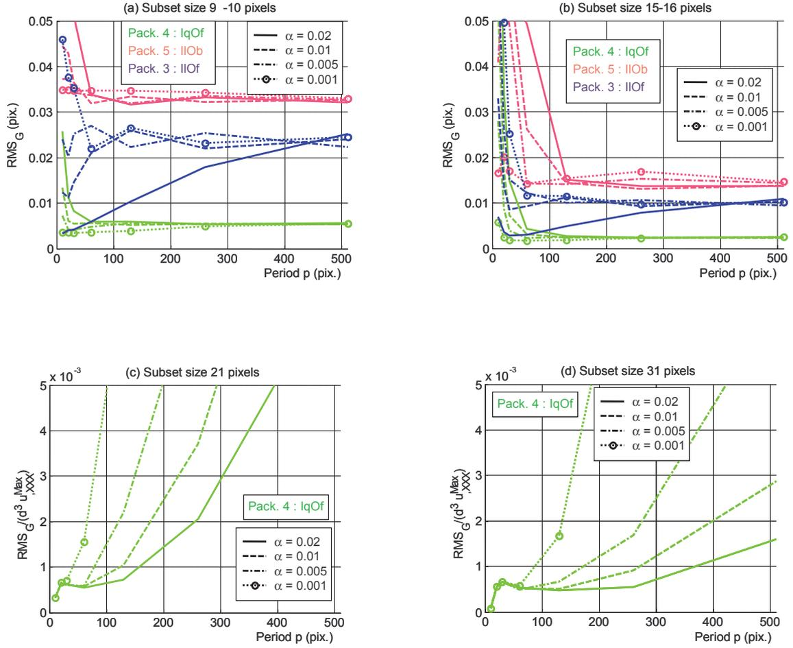
Figure 5:  $RMS_G$  as a function of period  $p$  for various strain amplitude  $\alpha$ , for a quadratic shape function and for three DIC packages. Subset size  $d$  is equal to 9 or 10 (a), 15 or 16 (b), 21 (c) and 31 pixels (d) respectively. The error is not normalized in (a) and (b), while it is divided by  $8\pi^3\alpha d^3/p^2$  in (c) and (d); only one DIC package is represented in (c) and (d).
