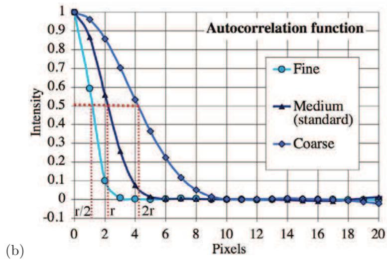
Figure 2: Illustration of synthetic speckle patterns. (a) fine, medium and coarse patterns and (b) associated centered and normalized autocorrelation function radius at half height.
