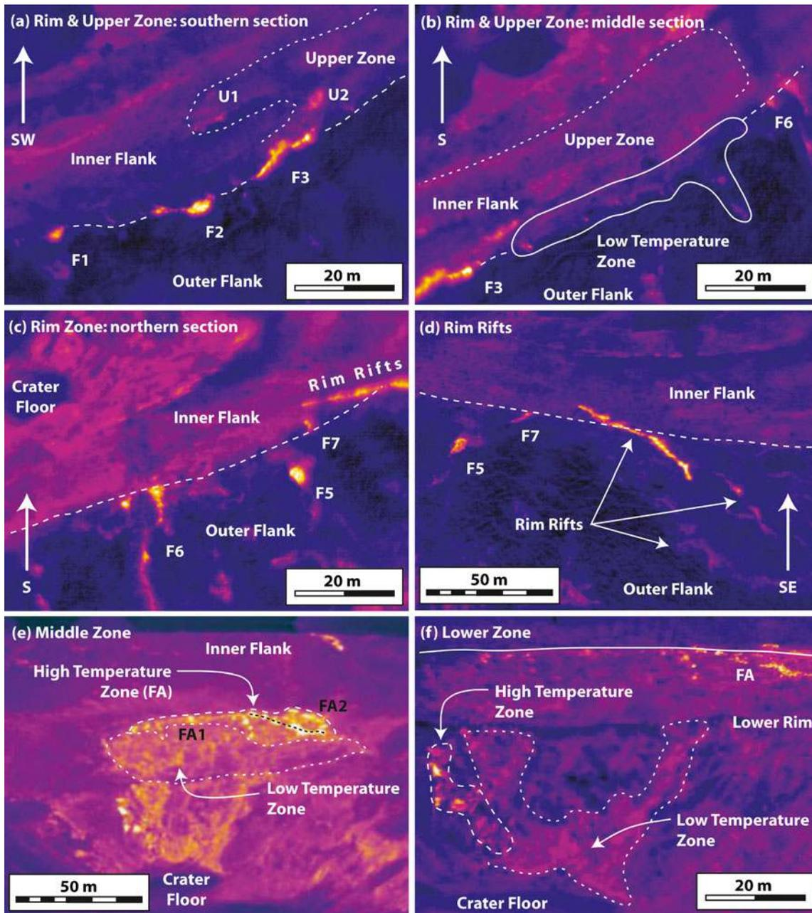
**Fig. 4** Thermal images of **a** the rim and upper zone (*southern section*), **b** the rim and upper zone (*middle section*), **c** the rim zone (*northern section*), **d** rim rifts, **e** middle zone and **f** lower zone. All images were acquired in 2005, where **a–d** are aerial oblique images acquired from a helicopter (*arrow gives view direction*). The main hot spots along the rim zone fracture are marked F1 through F7, and two hot spots
