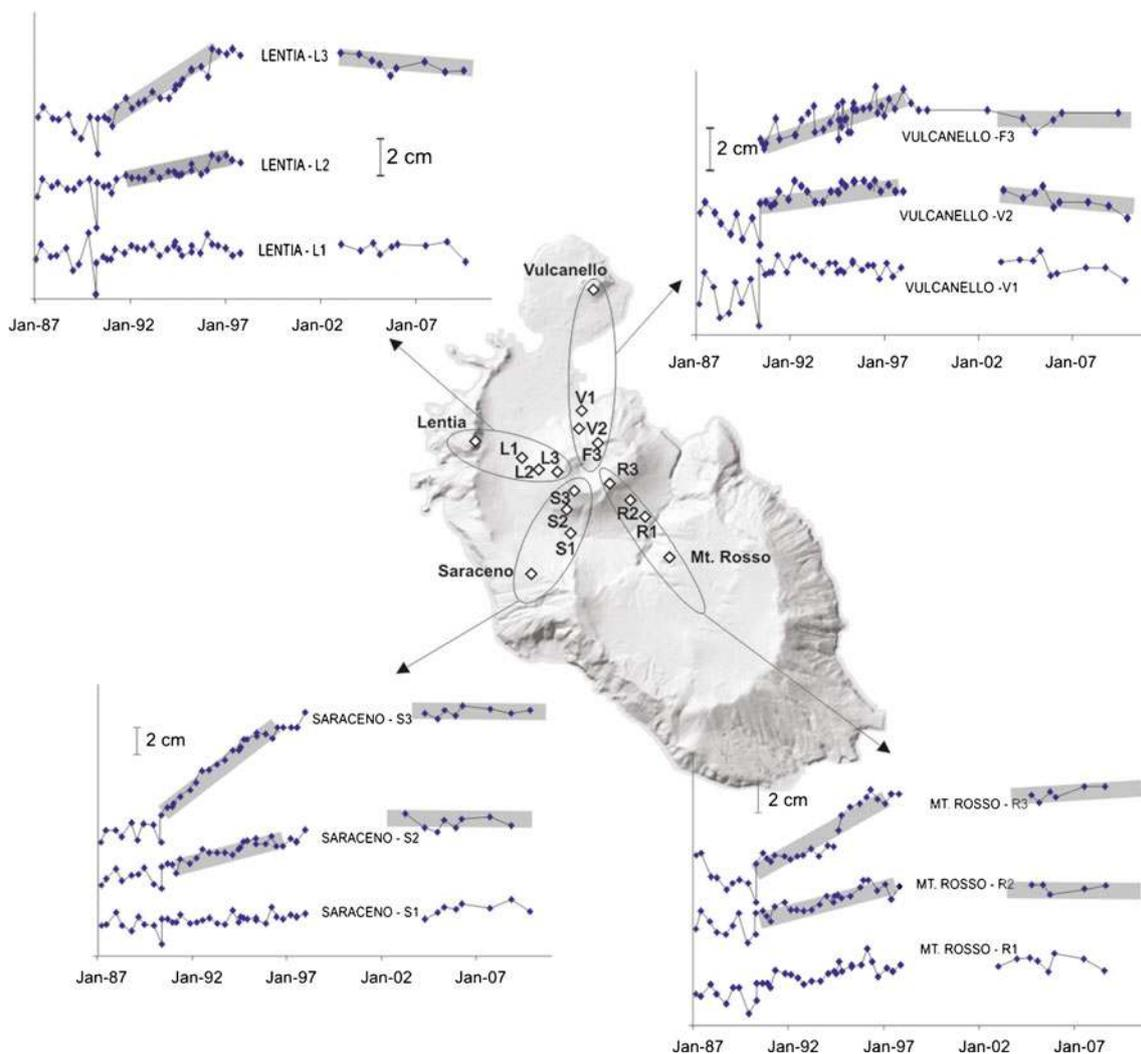
**Fig. 10** Changes in measured distance along lines connecting the benchmarks positioned on the Fossa cone and the stable benchmarks as function of time (1987–2009). Distance measurement errors are less
