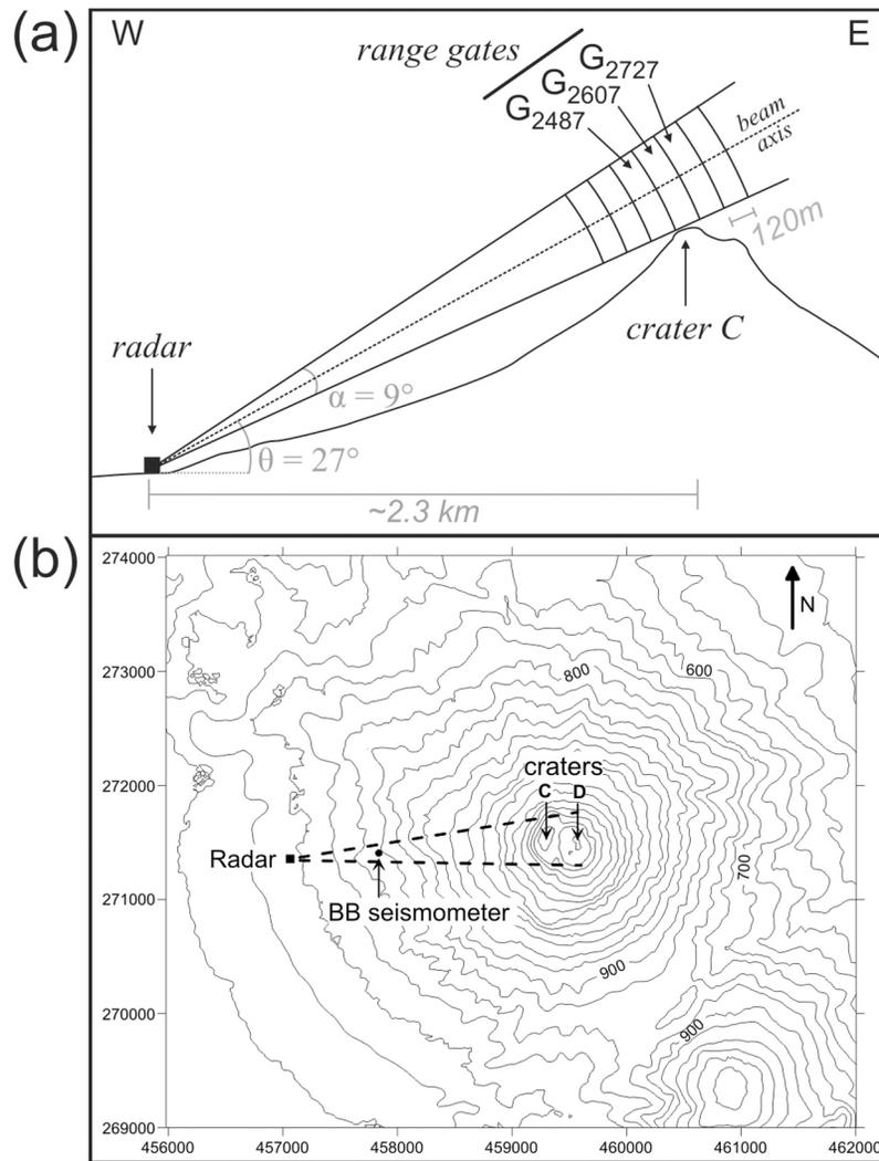
**Figure 1.** (a) Radar beam geometry during the recording campaign. (b) Location map of the broadband seismometer and Doppler radar. At the time of the recording campaign in February 2005, the estimated altitude of crater C is 1710 m above sea level (asl) [Wadge *et al.*, 2006].
