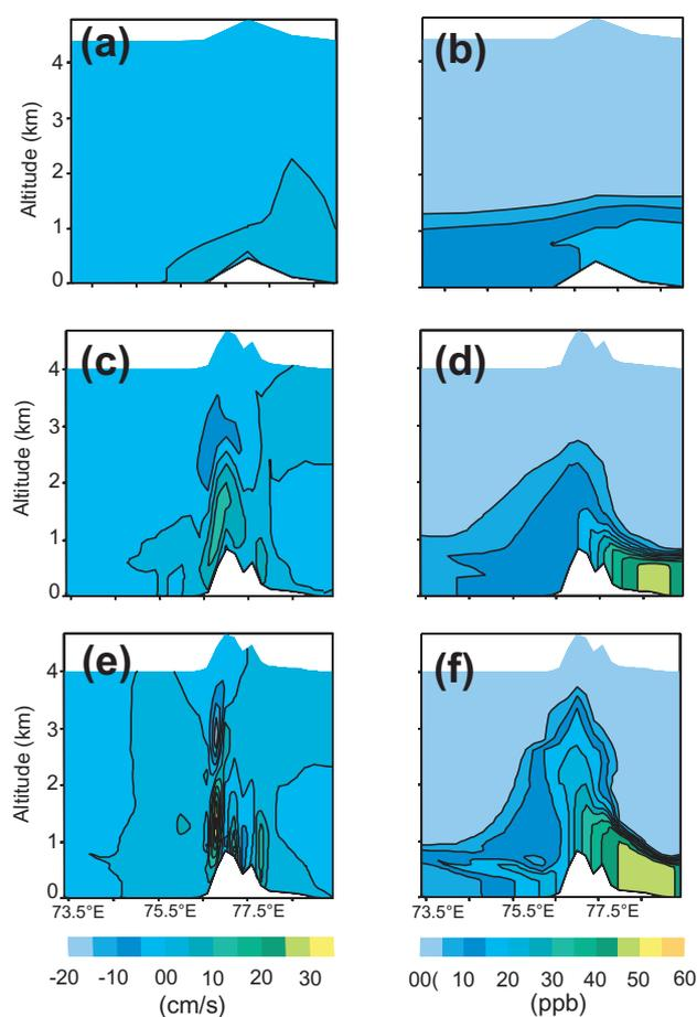
**Fig. 15.** Vertical distribution of the tracer concentration (ppb) and vertical velocity ( $\text{cm s}^{-1}$ ) at  $10^\circ\text{ N}$  latitude and between  $73^\circ\text{ E}$  and  $78.5^\circ\text{ E}$ , respectively, obtained with the 1-grid simulation (run A) referred to as S1 (a) and (b), with the 2-grid reference simulation (run B), referred to as S2 (c) and (d) and with the high resolution simulation (run C), referred to as S3 (e) and (f) at 12:00 UTC on 7 March 1999.
