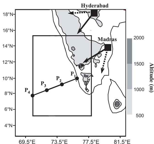
**Fig. 11.** Map of south India (with terrain elevation) and position of the 4 locations used to inspect the spatial and temporal structure of pollutants plume over the ocean: P1 (76.5°E; 10°N), P2 (74.3°E; 9.3°N), P3 (72.7°E; 8.6°N), P4 (69.9°E; 7.6°N). Dotted (solid) arrows represent the main wind direction before (after) 6 March 1999.
