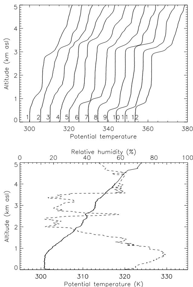
**Fig. 3.** (a) Potential temperature profiles obtained from dropsondes released from the Met Office C-130 Hercules aircraft on 7 March 1999 over the Arabian Sea between 05:19 and 07:34 UTC. (b) Potential temperature (solid line) and relative humidity (dotted line) profiles obtained with the 06:11 UTC balloon sounding launched in Kaashidhoo, Maldives.
