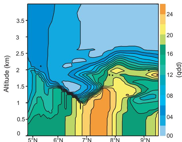
**Fig. 17.** Vertical distribution of the tracer concentration (ppb, all sources) along FT1 obtained with the sensitivity high resolution simulation on grid 3 (run C) at 03:00 UTC on 7 March 1999. The contours are obtained by summing the tracer fields from the four emission sources.
